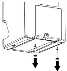
> Remove the cover from the rear of the device.
