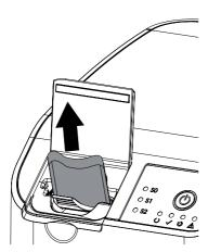
Once the image plate has been inserted into the unit, close the cover and leave it closed throughout the entire scanning process.
