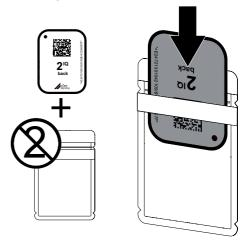
> Pull off the adhesive strip, fold down the flap and close the light protection cover tightly by pressing together firmly.
