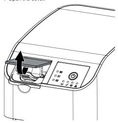
Place the light protection cover with the image plate centrally and straight onto the input unit. The torn-off side of the light protection cover faces down; the inactive (back) side of the image plate faces the operator.
